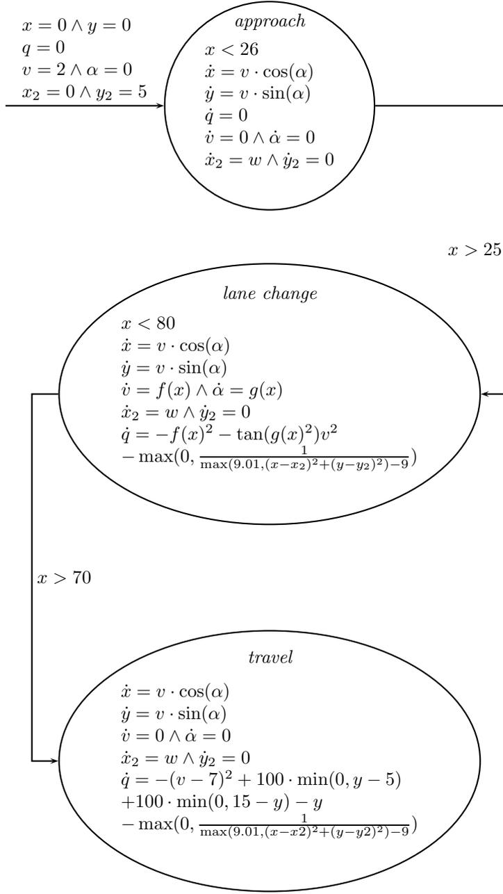
Figure 6: A model of a human driver moving onto a freeway with another vehicle already on the freeway.  $x, y$ : position,  $v$ : velocity,  $\alpha$ : angle to freeway direction,  $x_2, y_2$ : position of other vehicle,  $w$ : velocity of other vehicle,  $f \in [0, 2]^{\mathbb{R}}$ : acceleration (optimised function),  $g \in [-0.1, 0.1]^{\mathbb{R}}$ : steering (optimised function),  $q$ : reinforcement value (measured at  $x = 140$ )
