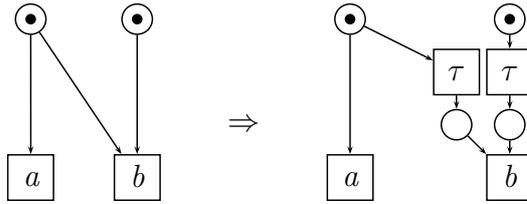
Fig. 1. Transformation to the symmetrically asynchronous implementation
